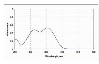
Tinuvin 326 exhibits strong absorbance in the 300 – 400 nm region and minimal absorbance in the visible region (> 400 nm) of the spectrum. The absorption maxima are at 312 nm and 353 nm ( $\varepsilon$  = 15600 l/mol·cm) in chloroform solution.
