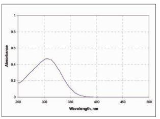
Uvinul 3039 exhibits high absorbance in the 280–320 nm region and no absorbance in the visible region (>400 nm) of the spectrum. The absorption maximum is at 306 nm in chloroform solution.
