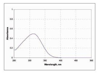
Uvinul 3030 exhibits high absorbance in the 280–320 nm region and no absorbance in the visible region (>400 nm) of the spectrum. The absorption maximum is at 311 nm in chloroform solution.
